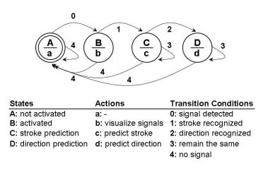
Figure 6. The state machine diagram.
