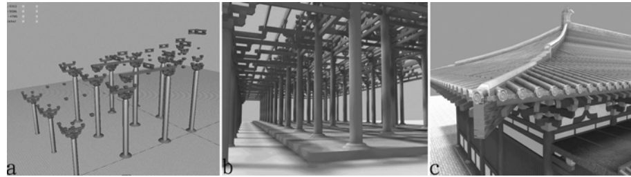
Figure 3: The process of computer modeling: (a) a structural framework, (b) its basic form, and (c) an integrated model.
