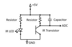
figure 2. Circuit scheme of homemade IR transceiver.
