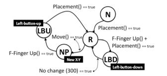
figure 5. Finite state machine for drag action.
