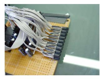
figure 3. Prototype of IR sensor bar.
